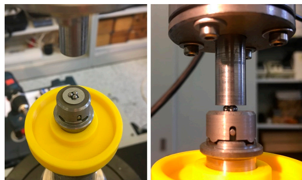
Figure 3. The test setup used for the measurements of the bi-axial flexural strength via B3B.
